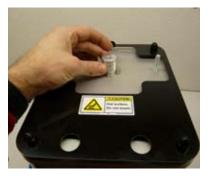
13. Place the flask onto the **myerson Flexpress**™, centering the sprue hole of the flask over the center of the heating chamber. Lock the flask in place using the flask strap and knobs.
